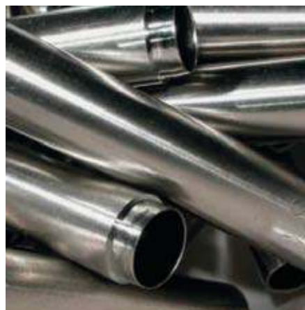
Fig. 1. Zirconium fuel rods for the nuclear industry.
