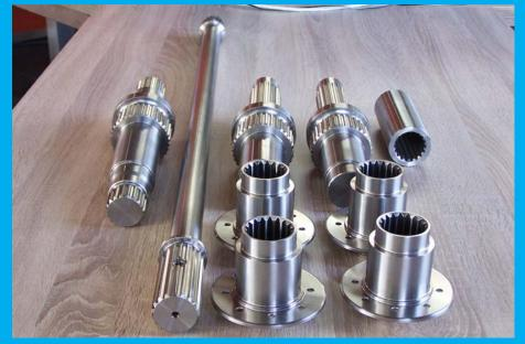
Titanium parts manufactured by Peekstok including a Ø70mm splined shaft. Photo: Peekstok
