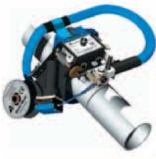
Picture 6. Open Servo Weld head. Universal standard open weld heads (with or without cold welding additive material) suitable for all diameters of tubing in excess of 20 mm.
