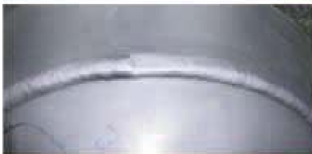
Picture 1. This fire-extinguishing pipe in 304L was apparently welded satisfactorily (see below), but the root penetration side (see above) was so bad that the pipe started to leak at these locations within a relatively short time.
