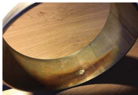
Figure 4: View of the inside of the MIC pierced 6" S10s size 316Ti pipe which had been filled with IJ river water. (photo: Innomet private company)
