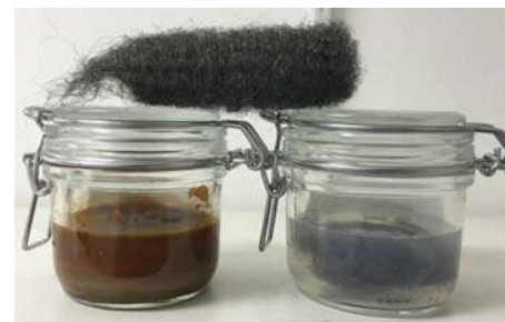
Figure 5: Test with PipeShield on steel wool: on the left is tap water, on the right tap water treated with PipeShield (photo: Innomet private company)
