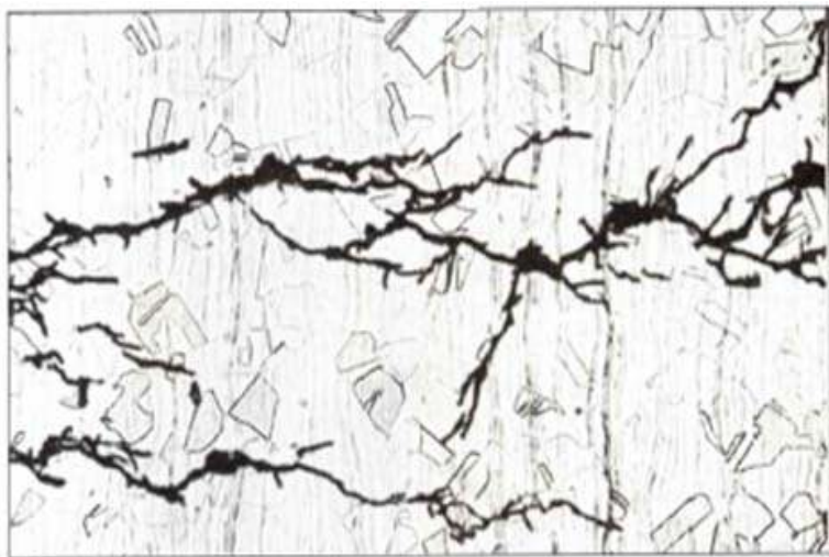
10. Trans-crystalline cracking caused by stress-corrosion
