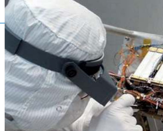
Mike Williams, a Lead Mechanical Engineer at the University of Arizona Lunar Planetary Lab, shown installing the structural manifold made of ATI 425 titanium on the Thermal Gas Evolved Analyzer (TEGA). TEGA is one of the instruments installed on the Phoenix Mars Lander. One of the key tasks assigned the Lander is to help determine whether microbial life ever existed on Mars.
