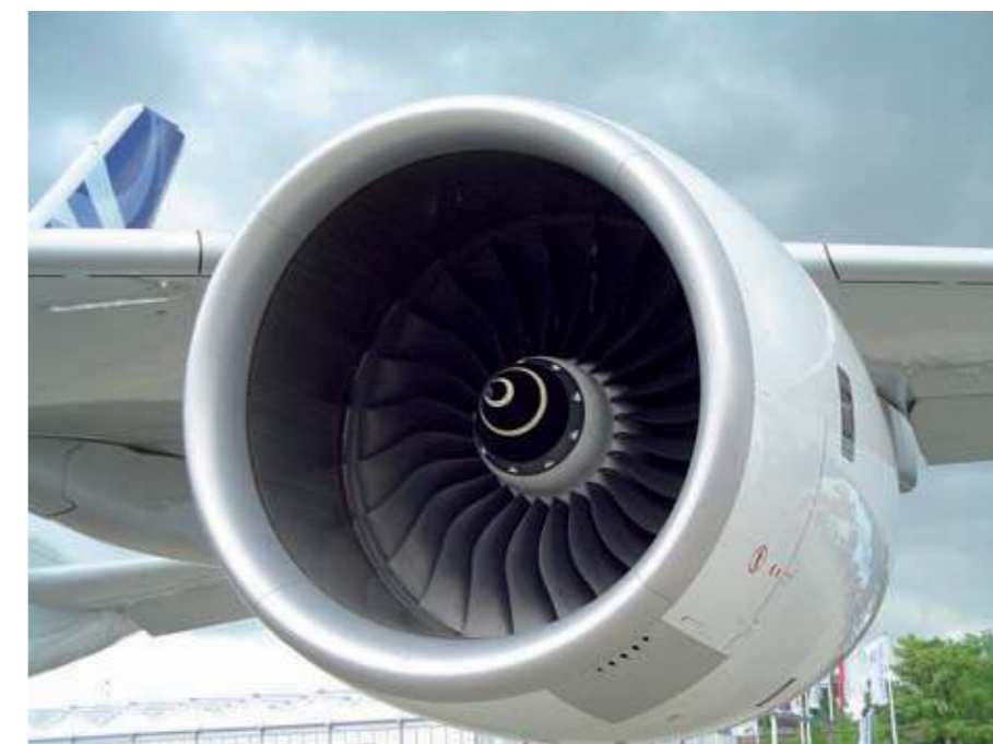
The engines alone of the Airbus A380 use about 11 tons of titanium.
