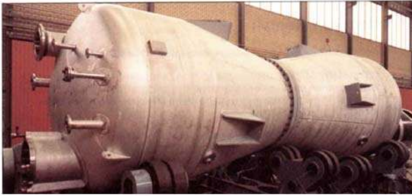
Composed reactors of 316L for the plastic industry
