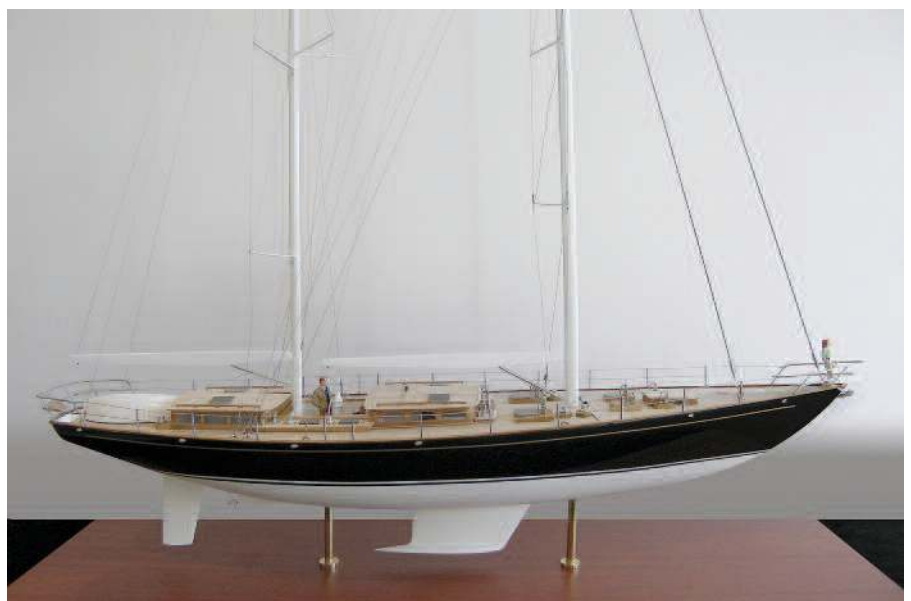
Fig. 7. The hull of this yacht is made from duplex stainless steel 1.4462 and fitted with intelligent anodes.
