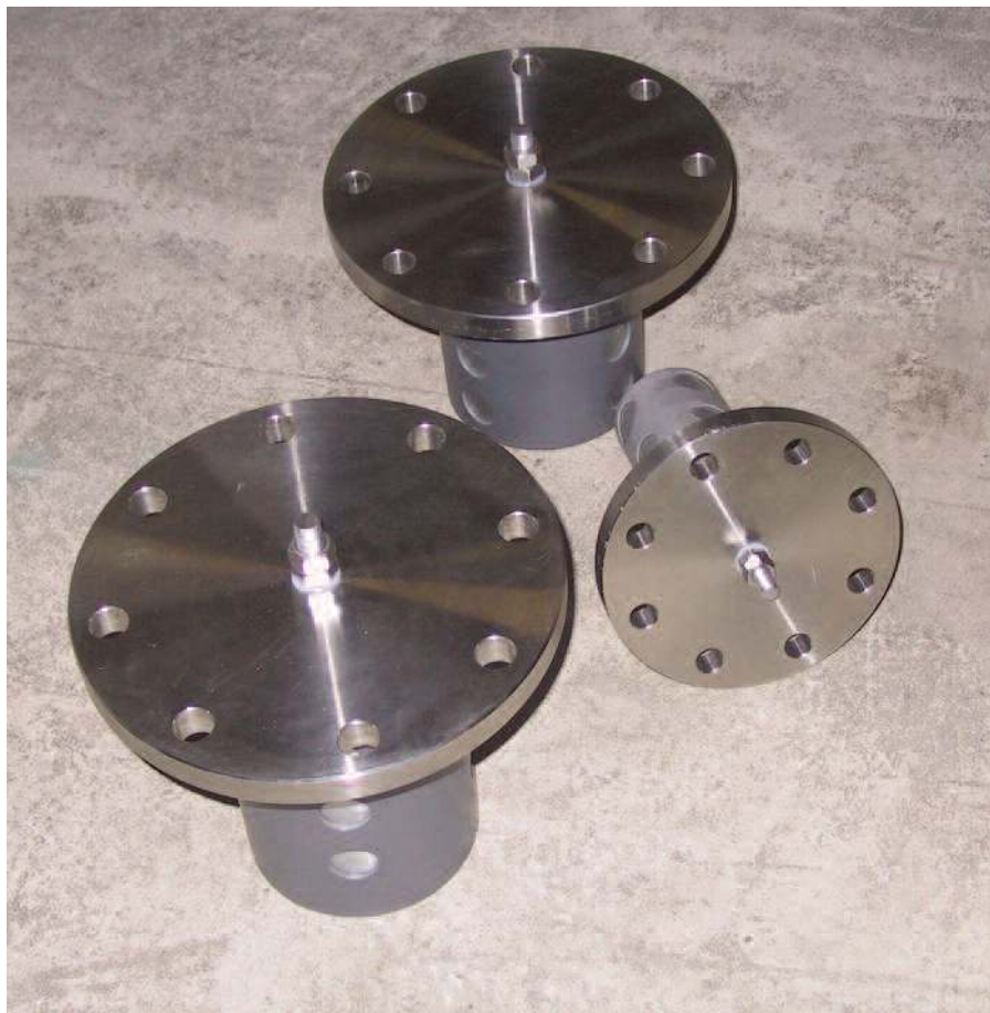
Fig. 4. Corrodium anodes with a stainless steel flange, used for seawater coolers etc. The electronic circuits are built in, eliminating the need for a separate housing or cables (photo by Corrodium B.V.).
