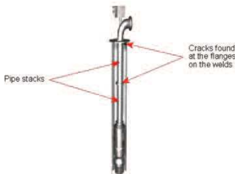
Fig. 5. A duplex seawater lift pump fitted with a riser.
